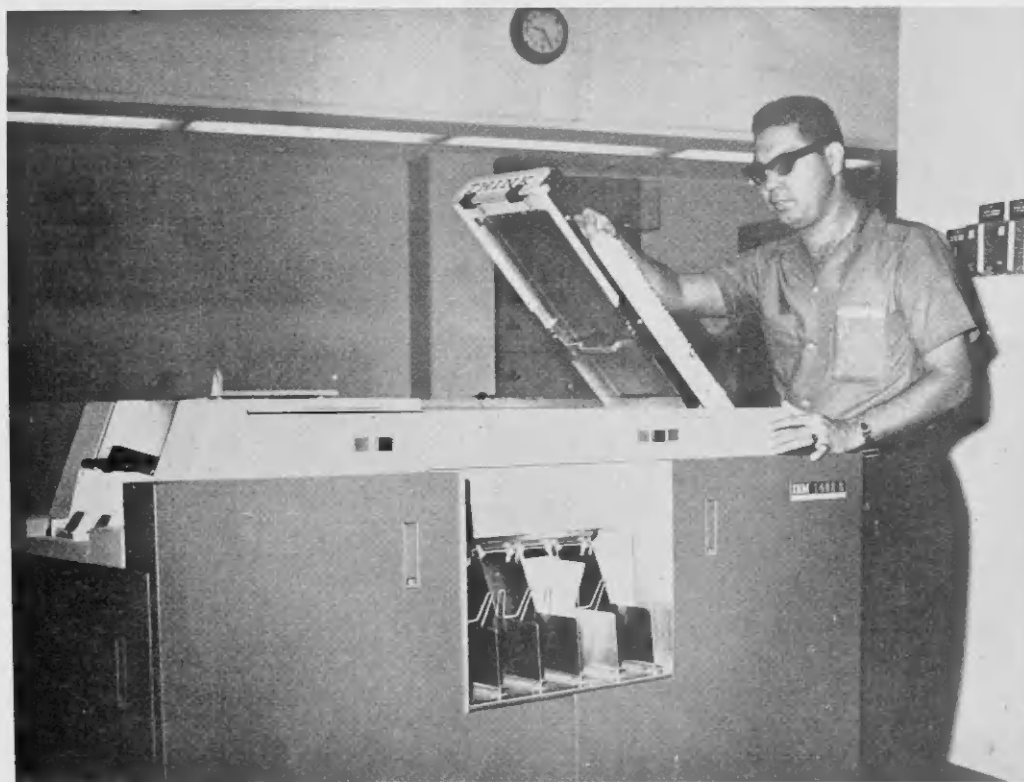
DATA CAN be read into the IBM 1402 reader-punch machine at the rate of 800 IBM cards a minute. Simultaneously, the unit can punch cards at the rate of 250 cards a minute with virtually no interruption of computing.
